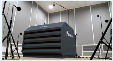
ound power level measurement in acoustic chamber
