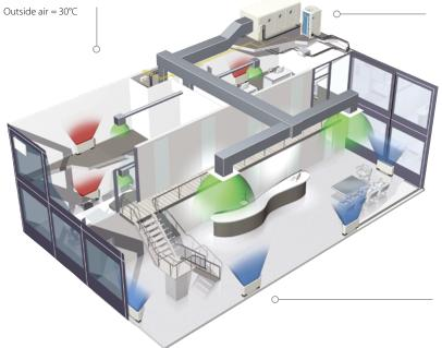
Fresh air AHU connected to VRV outdoor unit: The AHU takes care of the heat loads of fresh air securing air supply at 21°C.
