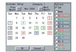
intelligent Touch Controller also offers yearly scheduling, error history and auto heating/cooling changeover functions, plus limits on set temperatures.
